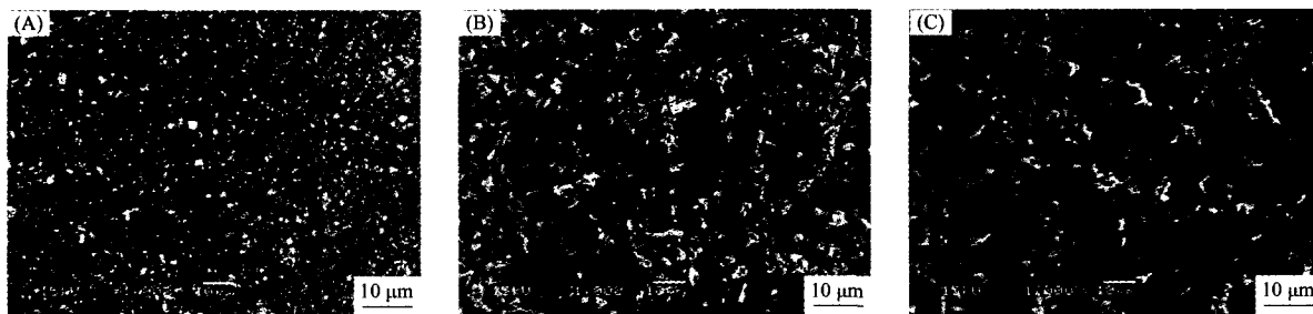
Fig. 1 SEM surface morphologies of ZnO films deposited at substrate temperature (A) 600 °C; (B) 650 °C; (C) 700 °C.
