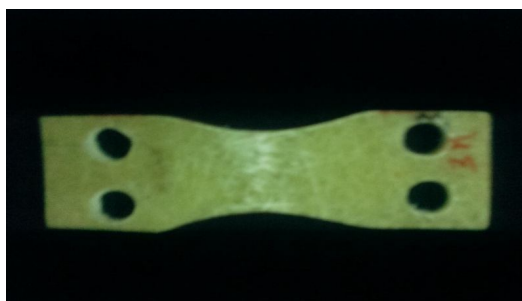
Figure 11 Photographs of tested specimens show damage resistance of 3% Vol. SiO 2 for nanocomposites reinforced 6 Layers of (CM) E-glass fiber.
